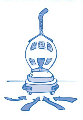
adon is a naturally occurring radioactive gas produced by the breakdown of uranium in soil, rock, and water. Air pressure inside your home is usually lower than pressure in the soil around your home's foundation. Because of this difference in pressure, your home acts like a vacuum, drawing radon in through foundation cracks and other openings.
